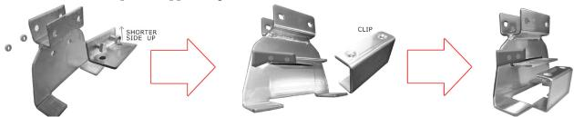
5. Attach the support and clip to the first and last tabs on each side of the van by pulling up and out on the clip and sliding it underneath each tab. *Note:* On models that have (4) tabs on each side, you will have to use the second tab in from the front of the van - not the first. Tighten the (2) 5/16°-18 x 1 hex head bolts pulling the clip and support together and clamping onto the tab. Repeat for additional supports.
