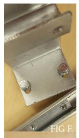
13. Once the channel are secured to the factory mounting positions, slide the threaded support tabs into position and secure the van rack support to the threaded support tab using (2) 5/16"-18 x 7/8" hex head bolts and (2) 5/16 split lock washers. Do not tighten completely at this point. FIG F.
