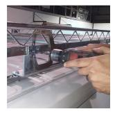
18. Using locking C-Clamps, clamp the van rack assembly to the pocket of the support. Do this to all support postitons. Once the van rack assembly is clamped into place, drill the holes in the square bottom tube of the side rails as designated by the pockets of the supports using a 5/16" drill bit.
