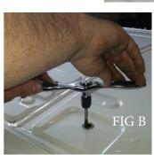
7. With the correct plugs on each side removed, clean the factory threaded with a M8 x 35 hand tap to remove any debris or paint chips that may impeed securing the channels to the factory mounting positions securely to roof of van. NOTE: Tap not included. FIG B.
